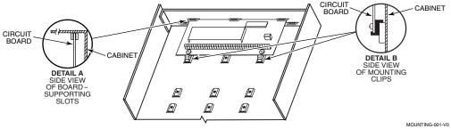
Figure 2. Mounting the PC Board
